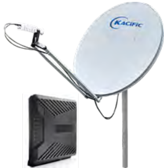
Kacific's terminal kit consisting of low power, high throughput ST Engineering iDirect MDM2010 IP Satellite modem, its paired iLNB 3210 transceiver, and the 1.2m VSAT antenna.
