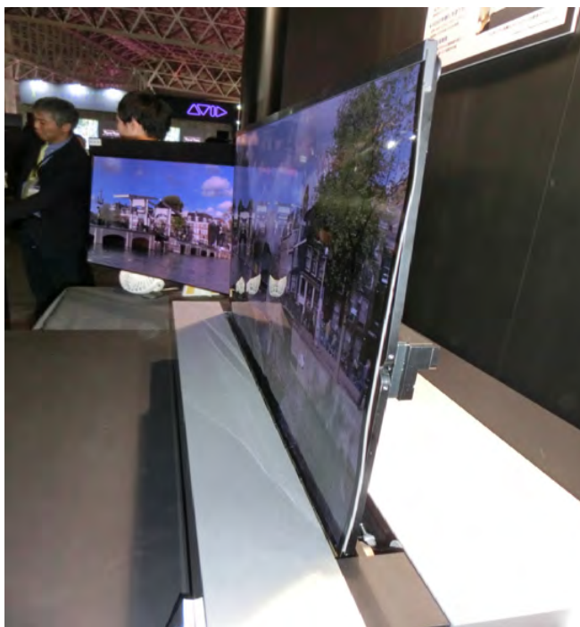
NHK unveiled for the first time in InterBEE 2019 a 30-inch 4K flexible OLED-based TV with 0.5mm thickness.
