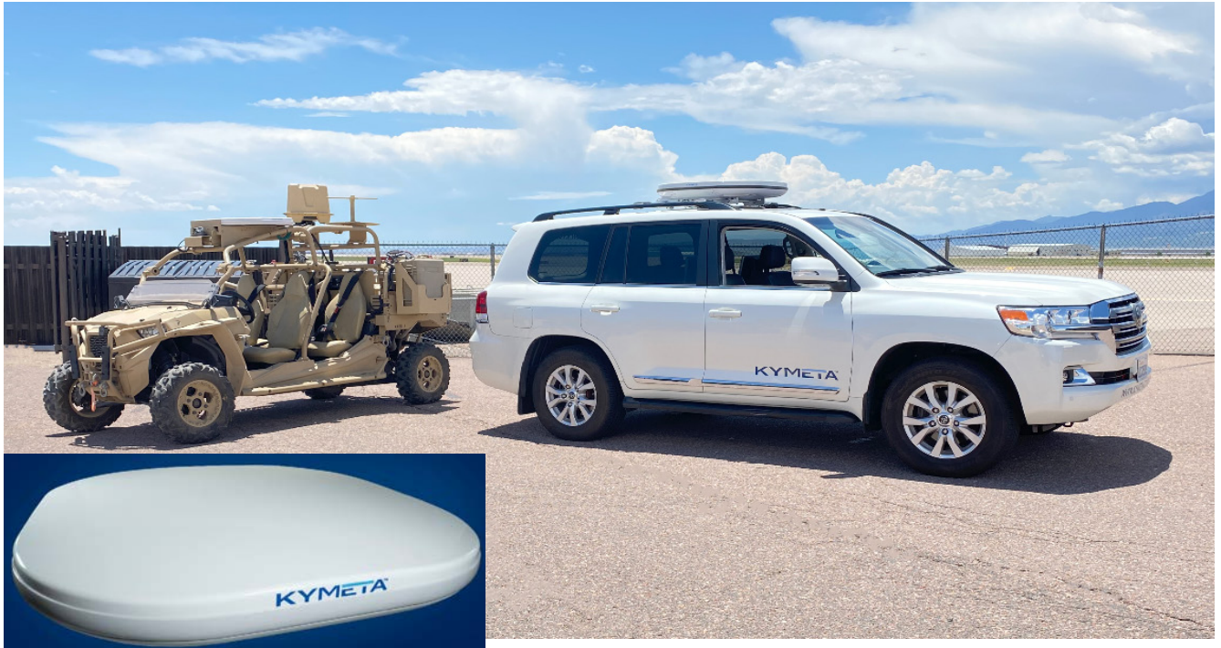
Kymeta's u8 terminal (inset photo) can be used for various COTM applications including military, government, public safety and commercial markets.
