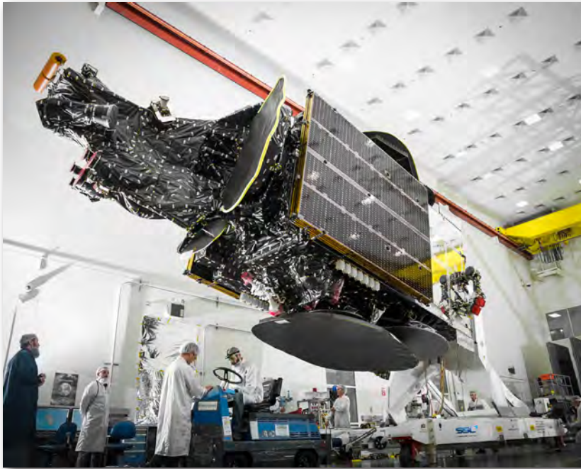
Manufacture of HTS satellites is rapidly rising with HTS capacity over oceanic regions growing almost 10-fold from 2017 to 2020. Photo shows Telstar 18 VANTAGE multi-mission satellite, built by SSL, for Telesat. Last month, SSL said the satellite has begun on-orbit operations. Photo Credit: SSL
