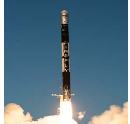
Firefly Aerospace's Alpha rocket designed to lift ~1,000 kilograms to a low earth orbit. (image courtesy of Firefly Aerospace)
