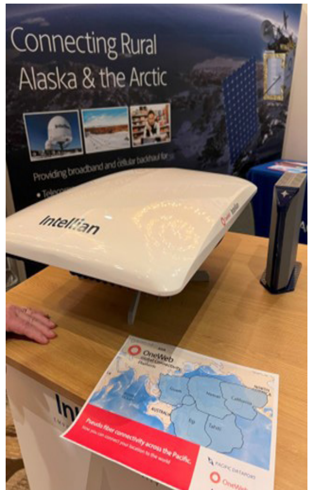
Intellian is working on flat panel antennas with separate surfaces for transmit and receive, on display at the PTC.(photo by Bruce Elbert)
